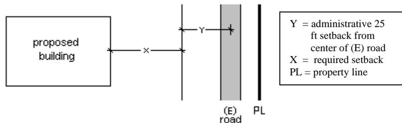
(4) Where a recorded easement exists, but roadway is located **outside of the easement**. In this case, the edge of the *administrative* easement takes precedence over the recorded one:
